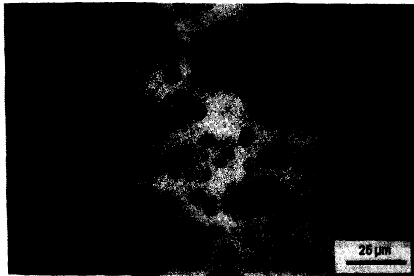
Fig. 6. CSLM image of a phase separated system containing 8.8% (w/w) Na-caseinate labelled with FITC and 2.0% Na-alginate in water. Note the presence of dispersed droplets in the dispersed phase (duplex system).
